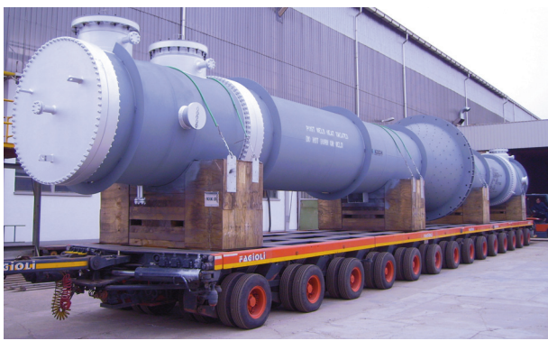
Figure 5. Reactor F/E TWISTED TUBE heat exchanger, Texas tower type, ready for shipment.
