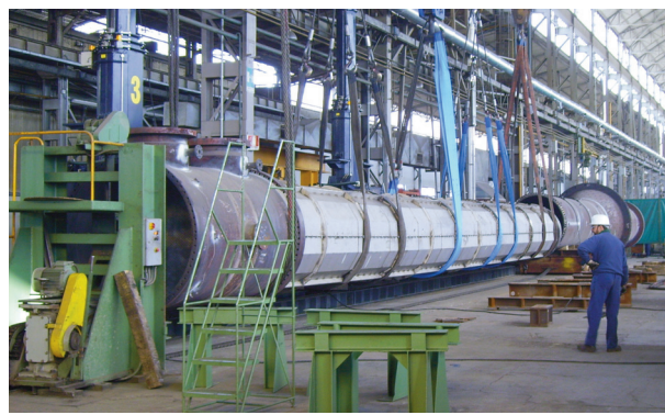
Figure 6. Insertion of the bundle in the Texas Tower heat exchanger at the production site.
